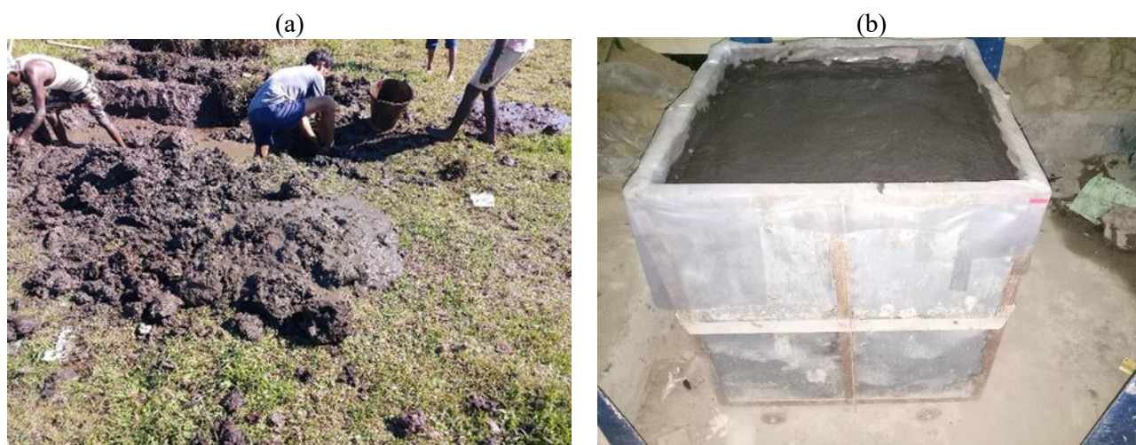
Figure 3. Peat samples were collected from the ETE site to conduct model-scale tests under controlled laboratory conditions. For accurate analysis, representative sampling was ensured by digging out the peat sample from a pit at the test location (a). The model test box (1 m × 1 m) was designed, constructed and prepared to simulate field conditions, with the peat surface 200 mm below the rim (b).
