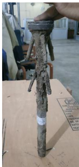
Figure 5. Top: Schematic diagram illustrating a model-scale BP installed in the tank, with labels identifying other components of the experimental setup (hydraulic jack, proving ring, load cell, LVDT). Middle: Photograph of the model-scale tank with key components of the setup in place. Bottom (from left to right): a casted BP in situ and three example BPs extracted from the peat after testing, with 4, 3 and 2 branches per whorl respectively. The extracted piles demonstrate remarkable alignment with the blueprint in terms of structural accuracy and experimental consistency.
