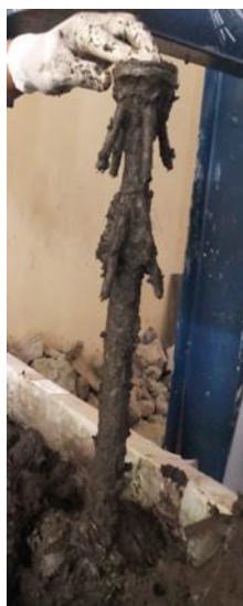
Figure 5. Top: Schematic diagram illustrating a model-scale BP installed in the tank, with labels identifying other components of the experimental setup (hydraulic jack, proving ring, load cell, LVDT). Middle: Photograph of the model-scale tank with key components of the setup in place. Bottom (from left to right): a casted BP in situ and three example BPs extracted from the peat after testing, with 4, 3 and 2 branches per whorl respectively. The extracted piles demonstrate remarkable alignment with the blueprint in terms of structural accuracy and experimental consistency.
