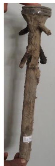
Figure 5. Top: Schematic diagram illustrating a model-scale BP installed in the tank, with labels identifying other components of the experimental setup (hydraulic jack, proving ring, load cell, LVDT). Middle: Photograph of the model-scale tank with key components of the setup in place. Bottom (from left to right): a casted BP in situ and three example BPs extracted from the peat after testing, with 4, 3 and 2 branches per whorl respectively. The extracted piles demonstrate remarkable alignment with the blueprint in terms of structural accuracy and experimental consistency.
