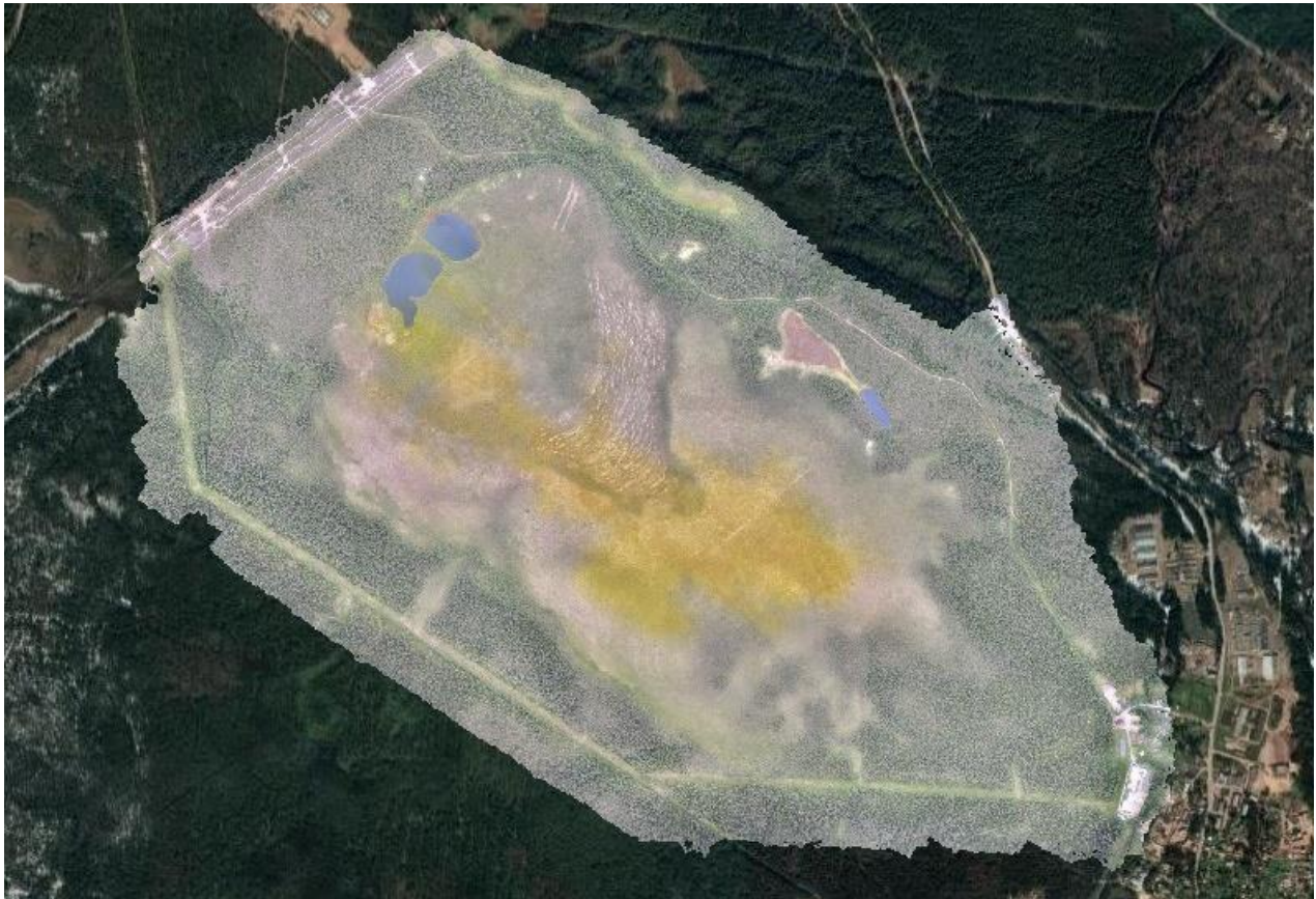
Figure A1. Orthomosaic map of the Lammin-Suo mire by Edward Kazakov, 03 Sep 2019. The light area indicates extent of the survey, and yellow spots possible defects resulting from different lighting conditions.
