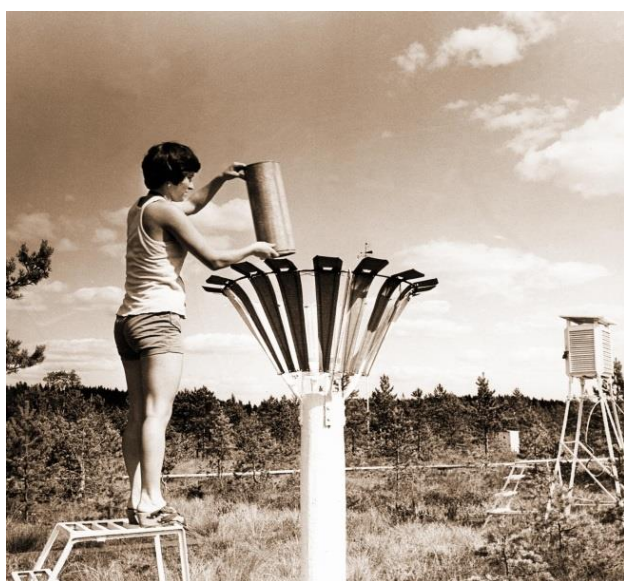
Figure 7. The Tretyakov precipitation gauge at Bolotnaya station in 1960 and 2021.
