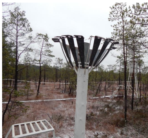
Figure 7. The Tretyakov precipitation gauge at Bolotnaya station in 1960 and 2021.
